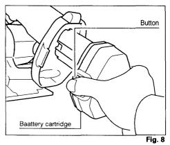
•Do not use force when inserting the battery cartridge. If the cartridge does not slide in easily, it is not being inserted correctly.
